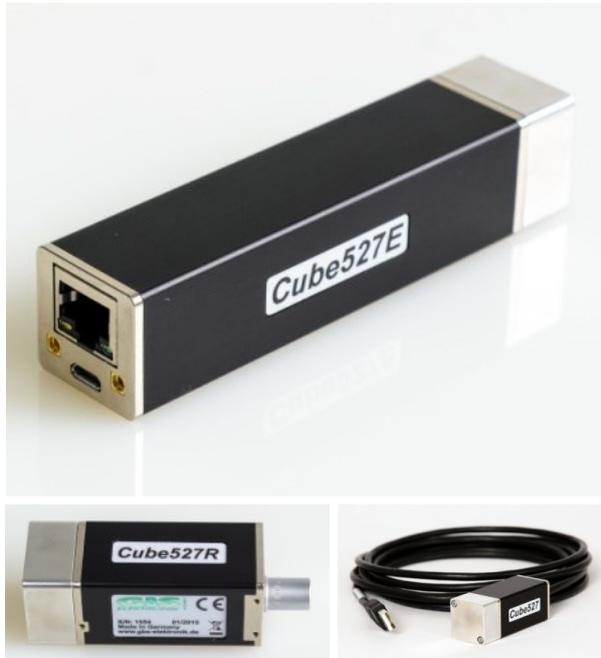
computer connection. The Cube527 is powered from the USB interface port, or by “Power over Ethernet“. Furthermore, we offer fixed cable versions for each computer interface version. Due to the integration of all hardware components which are required for a full gamma spectroscopy system in one package, only one cable is necessary to connect the system to a computer or network switch. The Cube527 series can be operated with our free of charge software programs, such as WinSpec or WinMCS.
